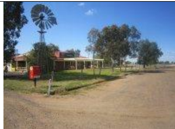
24. Public Posting Box is not accessible. A hard-stand area, with circulation space 1540 mm X 2070 mm, is required in front of the posting slot.
